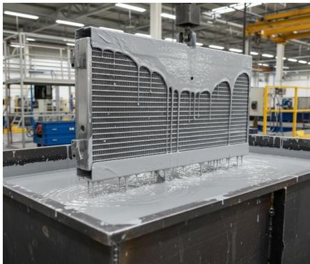
It is ideally suited for Radiator DIP (Immersion) Coating, where bundles of radiator fins—typically made of steel or aluminum—are immersed into a coating tank containing the primer.
